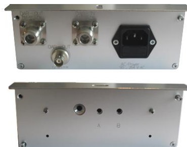
⌞ Standard (Master) Repeater VPRS ⌘ VPRS Repeater (additionally with heat sink, without fan)
