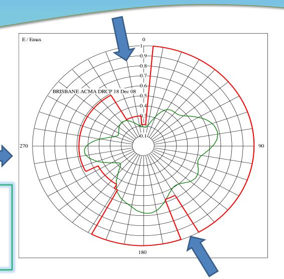
RF network design must consider interference and well as coverage
